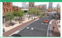
A separated route specifically for cycles that runs alongside a road or street. It is distinguished by vertical barriers, coloured asphalt/paint and/or elevation differences.
