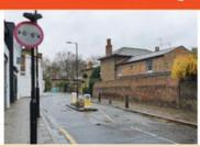
Physical design (e.g. lane narrowing, speed bumps) and psychological measures (e.g. different surface material) which encourage motorists and cyclists to slow down along a specific section of road.
